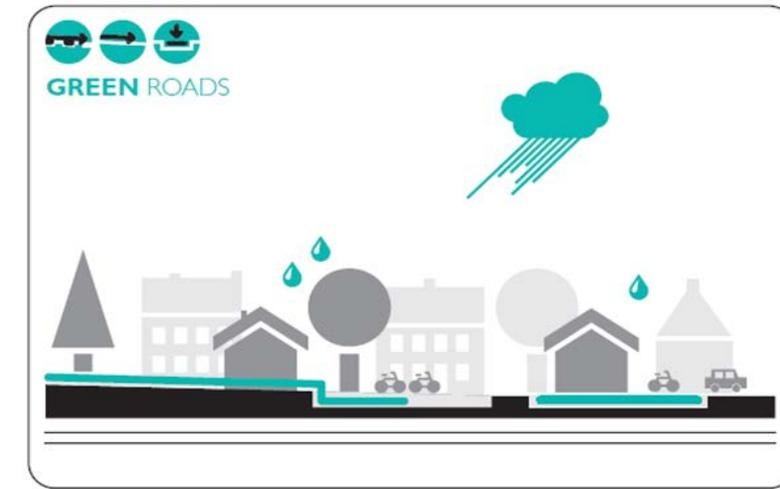
The hydraulic function of green roads is to remove and retain the water locally, typically on smaller roads, for example private shared roads.
