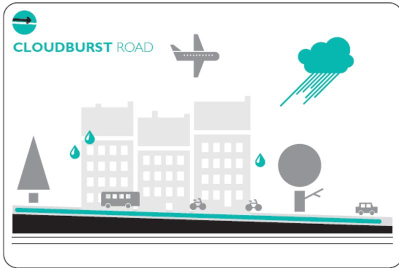
The principal hydraulic function of cloudburst roads is to discharge water. Cloudburst roads are established by re-profiling the road, making changes to terrain or raising the kerb. In principle, no green elements are incorporated in a cloudburst road.
